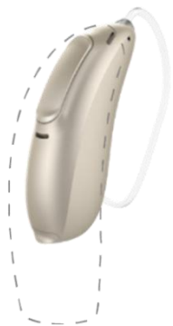
Figure 2. Image showing an Audéo M-312 overlaid on an Audéo B-13 with Roger 18 design-integrated receiver.
