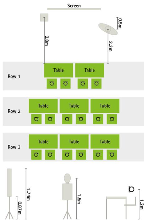
Figure 1. Experimental setup for impulse response measurements in the KAS in Hörzentrum Oldenburg.
