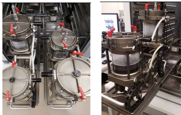
Figure 1: Test setup of the seawater and pool water dive test in climate-controlled chambers.
