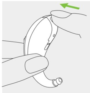
The battery is only secured when the battery door is closed correctly. Always check after closing, that the battery door cannot be opened by hand.
