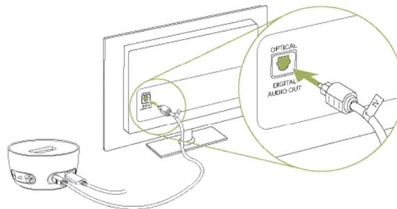
ⓘ Protect your eyes of the optical light from the optical Toslink cable when plugged into the device or TV.
