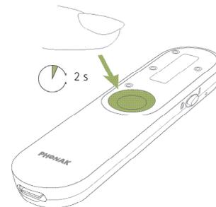
The muted microphone is indicated by a crossed microphone and crossed radio icon on the display. This means, that your microphone does not transmit a radio signal and your hearing aid may switch back into the automatic program. To unmute the microphone again, press and hold the function button again for two seconds.
